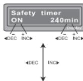
When you start a charge process, the integral safety timer automatically starts running at the same time. This is programmed to prevent overcharge the battery if it proves to be faulty, or if the termination circuit cannot detect the battery full. Please refer the statement in below to calculate the time setting.
